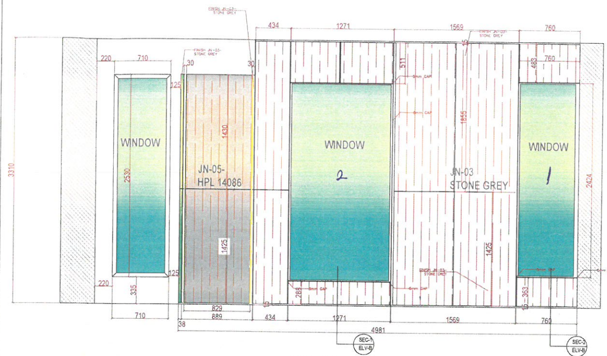
FRONT VIEW-B RECEPTION CLADDING
