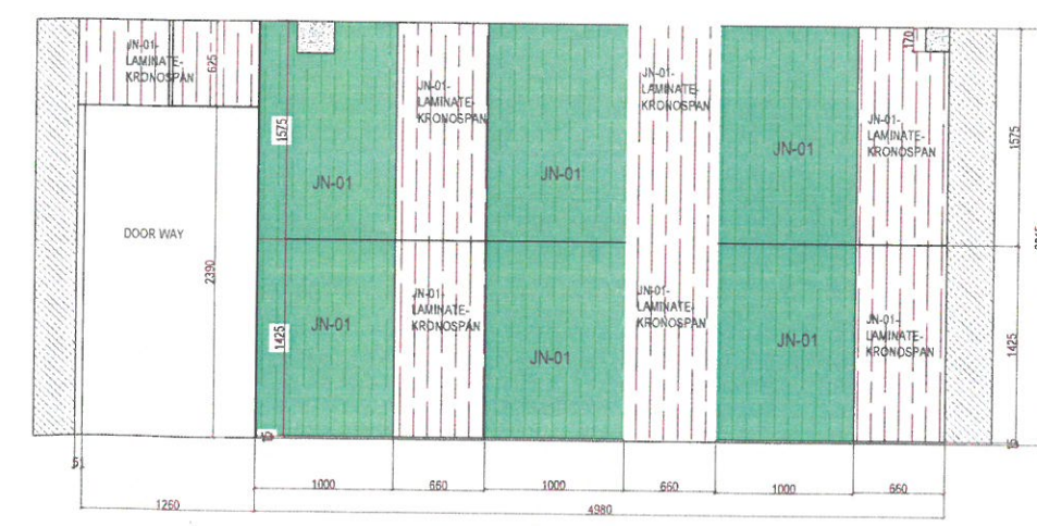
FRONT VIEW-D RECEPTION CLADDING
